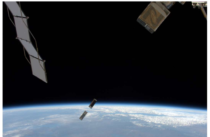
Astronaut Tim Peake on board the International Space Station captured this image of a CubeSat deployment on May 16, 2016. The bottom-most CubeSat is the NASA-funded MinXSS CubeSat, which observes soft X-rays from the sun—such X-rays can disturb the ionosphere and thereby hamper radio and GPS signals. (The second CubeSat is CADRE — short for CubeSat investigating Atmospheric Density Response to Extreme driving - built by the University of Michigan and funded by the National Science Foundation.) Credit: ESA/NASA
