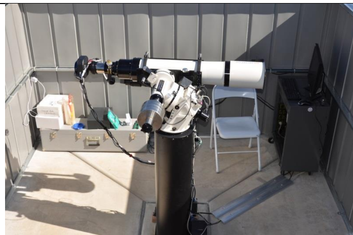
Figure 11- Scope Mounted and Wiring in Place
