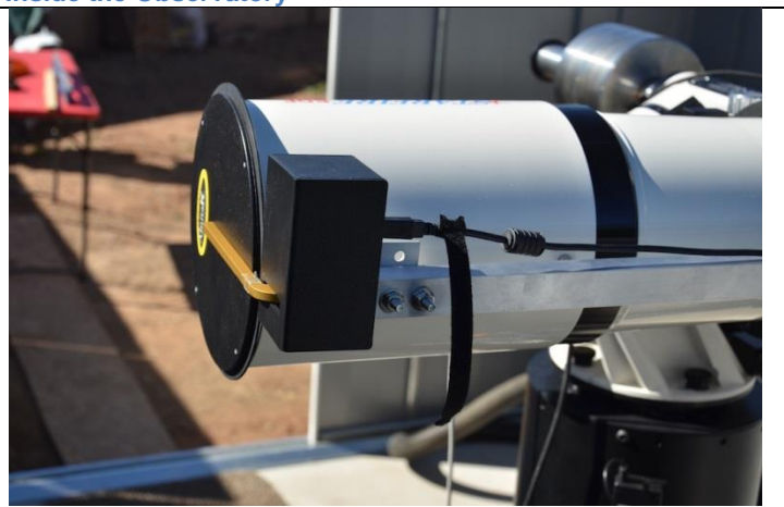
Figure 12- Flip Flat as a Dust Cover on a Homemade Rail
