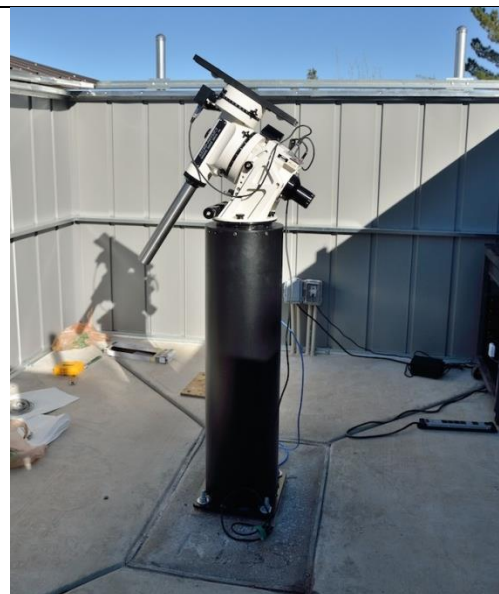
Figure 9- AP900 Mount Installed
